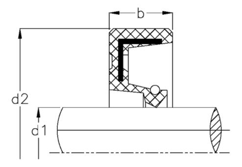
$\begin{array}{ll} b & = 7 \\ d1 & = 14 \\ d2 & = 26 \\ Material = NBR \end{array}$
